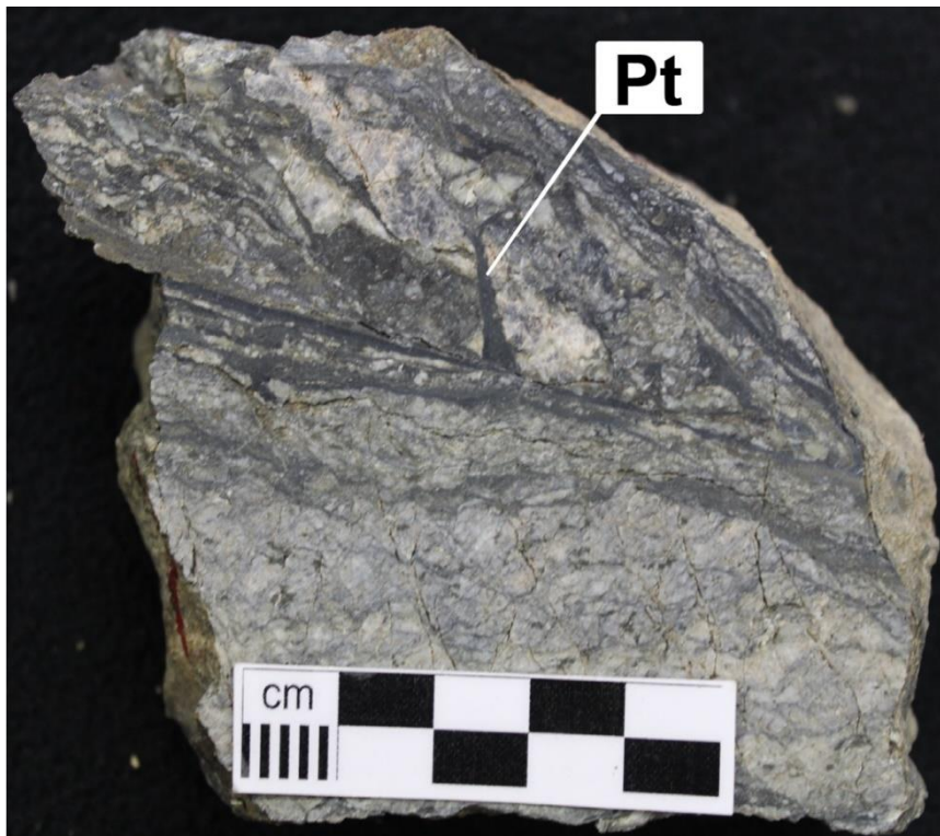
Figure 1: Pseudotachylite veins ('Pt') crosscutting paragneiss of the Austroalpine basement along the Pustertal-Gailtal Line (locality: Maria-Luggau, Lesachtal, Austria).
